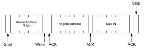
Figure 7-7 : example of a 2-wire write operation
