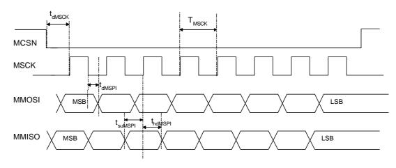
Figure 7-4 : SPI master interface timing, here is shown a one byte transaction.
