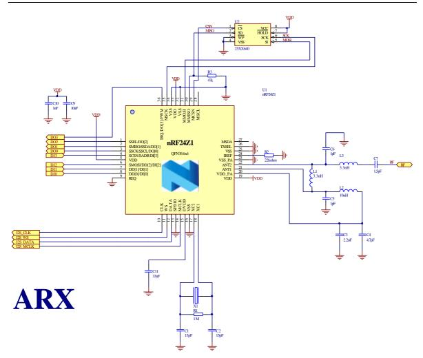
Figure 17-2 nRF24Z1 ARX with SPI EEPROM schematic
