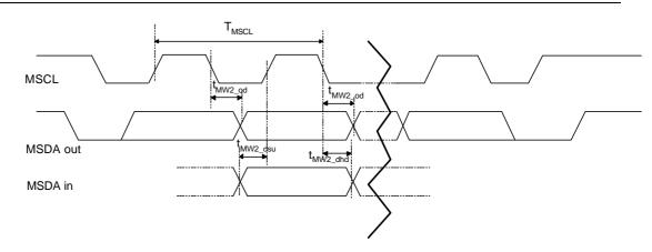
Figure 7-6 : 2-wire master timing, for values see Table 13-1
