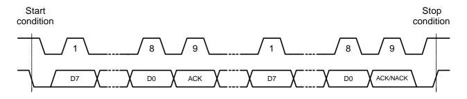
Figure 7-9 : example of 2-wire waveform
