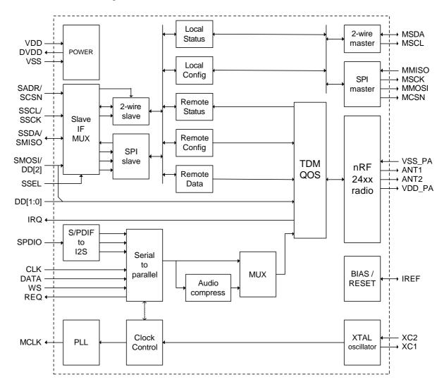
Figure 4-2 nRF24Z1 ATX mode block diagram
