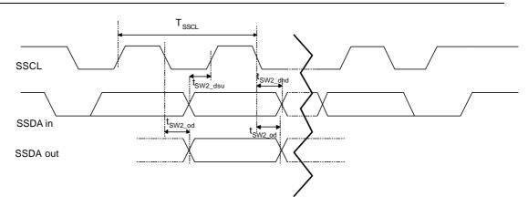
Figure 7-11 : 2-wire slave timing diagram, for values see Table 13-1
