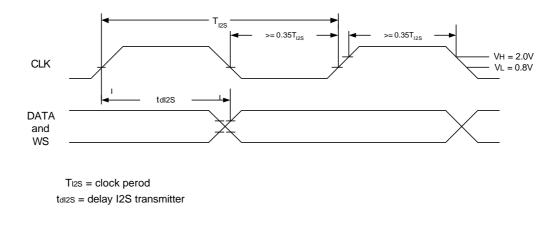
Figure 7-3. Timing for I2S output of nRF24Z1, for values see Table 13-1
