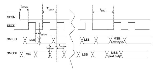
Figure 7-10 : SPI slave timing diagram
