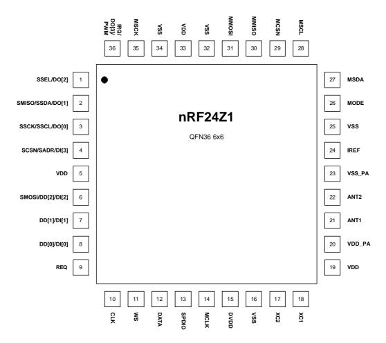
Figure 1-1: Pin assignment nRF24Z1
