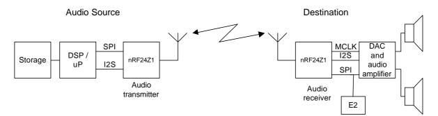
Figure 4-1 Typical audio application using nRF24Z1
