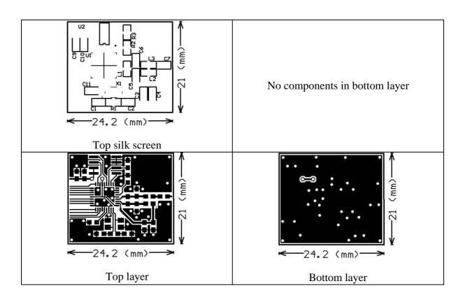
Figure 17-4 : nRF24Z1 ARX PCB layout
