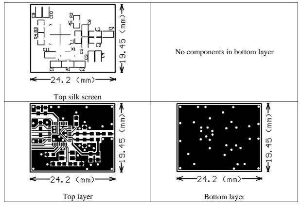
Figure 17-3 : nRF24Z1 ATX PCB layout
