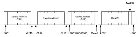
Figure 7-8 : example of a 2-wire read operation
