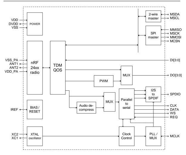
Figure 4-3 nRF24Z1 ARX mode block diagram
