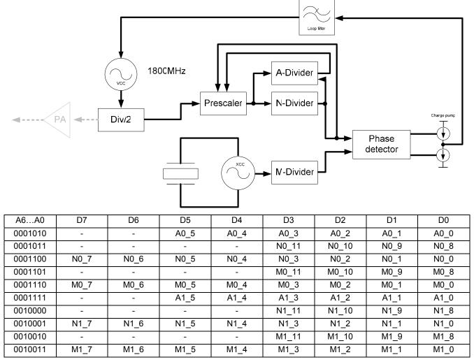
The lengths of the N, M, and A registers are 12, 12 and 6 respectively The values can be calculated from the following formula:
