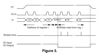
In the figure, 1 register is read. The address is A6, A5, ... A0. A6 = msb. The data read out is D7, D6, ...D0. The value of the R/W bit is always "1" for reading.
