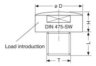
These load buttons prove extremely useful if a mechanical coupling (for instance, by means of a threaded rod) is not necessary or possible for a measurement of compressive forces. The spherical surface minimises measurement errors in case of not axial force introduction. The compression force needs to be introduced into the load button by means of a component with a plane surface, hardness  $\geq$  60 HRC.
