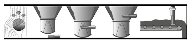
Typical installation positions for a moisture sensor.
