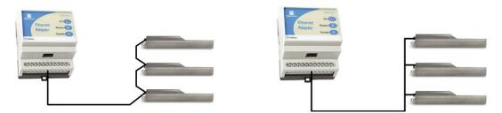
Figure 31: Correct RS485 cable network
