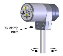
Figure 14: Adjusting the sensing head angle
