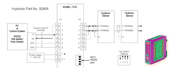
Figure 26: RS232/485 converter connections (0049A)
