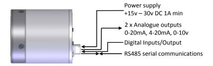
Figure 2: Connecting the sensor (overview)
