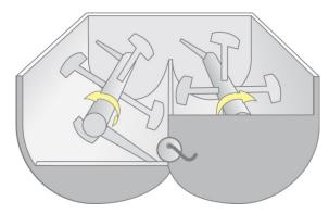
Figure 9: Hydro-Mix installed in an organic material mixer
