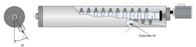
Figure 11: Hydro-Mix installed in a screw conveyor
