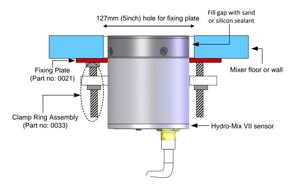
Figure 15: Sensor installation
