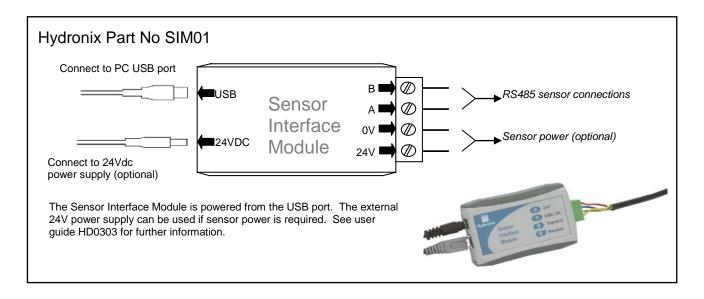
Figure 27: RS232/485 converter connections (SIM01A)
