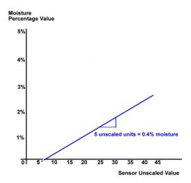
Figure 37: Gradient of unscaled values to moisture percentage
