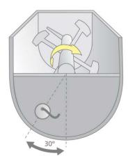
Figure 10: Hydro-Mix installed in a Single shaft mixer
