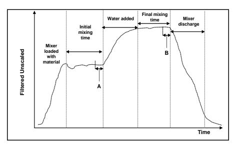
Figure 32: Typical moisture curve
