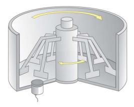
Figure 5: Position of sensor in a turbo mixer
