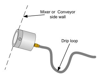
Figure 14: Hydro-Mix installed with a drip loop
