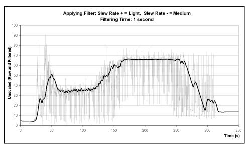
Figure 34: Filtering the RAW signal (1)
