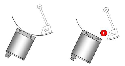
Figure 4: Mounting in a curved surface
