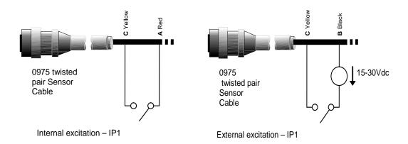
Figure 31: Internal/external excitation of the digital input
