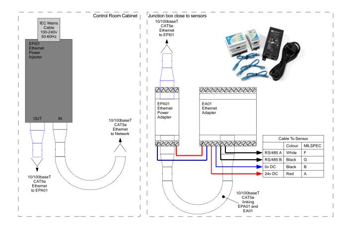
Figure 29: Ethernet Power Adapter Kit connections (EPK01)
