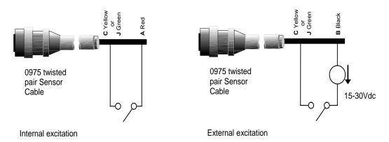
Figure 23 - Internal/external excitation of digital input 1 & 2
