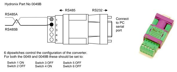
Figure 25: RS232/485 converter connections (0049B)
