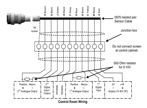
Figure 20: 0975 Sensor cable connections
