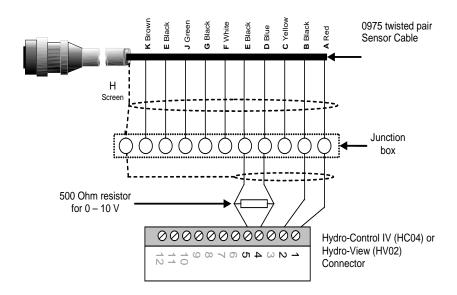
Figure 22: Connecting to a Hydro-Control IV or Hydro-View
