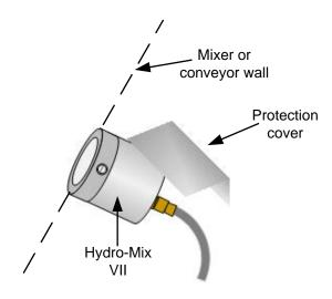
Figure 13: Hydro-Mix with deflector plate installed
