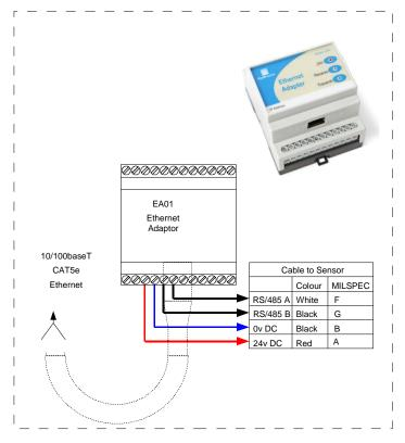
Figure 28: Ethernet Adapter Connections (EAK01)
