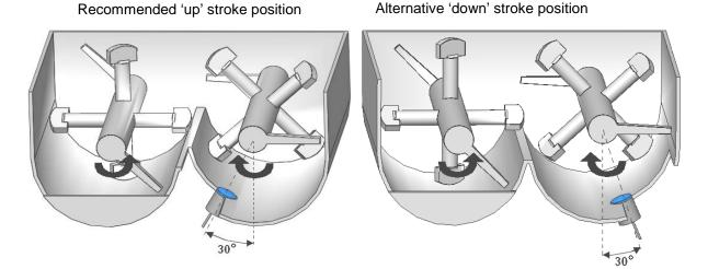
Figure 8: Position of sensor in a twin shaft horizontal mixer
