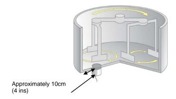
Figure 6: Position of sensor in a planetary mixer
