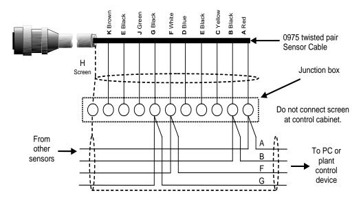
Figure 21: RS485 multi-drop connection
