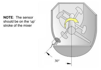
Figure 7: Position of sensor in a horizontal shaft or ribbon mixer
