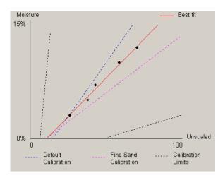
**Moisture % vs. Unscaled Calibration Graph**: The calibration data is displayed in a graphical form together with two default sand calibrations and the maximum and minimum calibration slopes defined by Hydronix, see Appendix A for more information.
