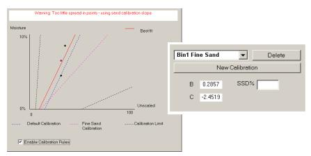
If for this same data set, the calibration rules are disabled, the graph changes to exclude all the dashed lines and the calibration line is drawn as a mathematical best fit line. No warning message is given and the resultant calibration coefficients are included for comparison below.
