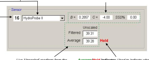
Live 'Unscaled' readings from the selected sensor, required for the material calibration. For more information on these readings, see appendix B. Average/Hold indicator: Used to indicate when batch averaging is taking place. This can be either from the digital input or remote averaging. When this changes to Average, the filtered unscaled is currently being averaged. When averaging is finished the 'Average' unscaled value is held constant and the label changes to Hold.
