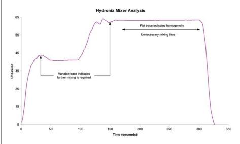
Figure 5: A typical mix cycle as seen by a Hydronix mixer sensor (Hydronix data)
