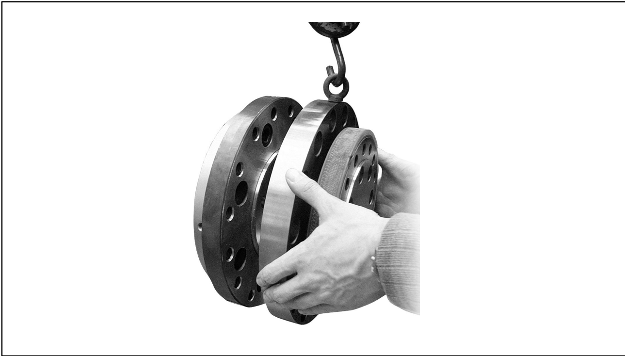
Fig. 4.3: Rotor installation (horizontal)
