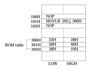
Specifying a ROM table address of 300H and a comparison value of 33H produces a break one instruction after the MOVLB [HL],300H instruction at address 101H, that is, after the NOP instruction at address 102H.
