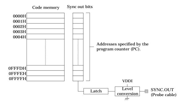
Figure 2-14 Sync Out Bits
