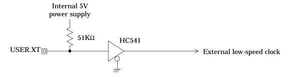
The user cable low-speed clock (USER.XT) input uses the emulator's internal operating voltage (5 V) for its "H" level.
