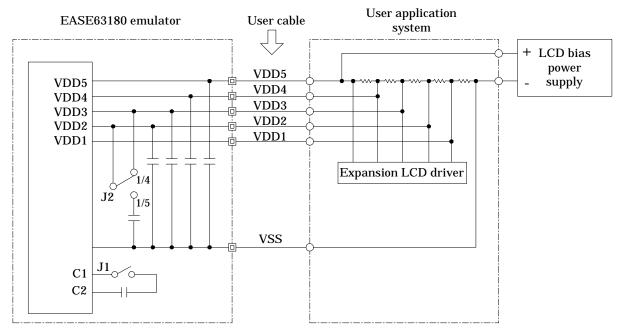
Figure 3-3 Interface Example for Expansion LCD Driver with External Bias Power Supply
