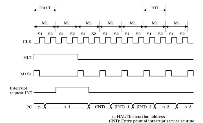
Figure 4-4 Halt Mode Timing Chart
