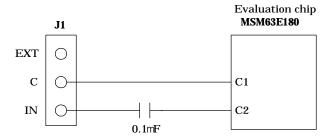
Figure 2-20 Jumper 1 Circuit
