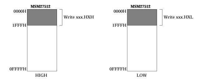
Figure 2-1 Address Ranges for MSM27512
