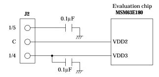
Figure 2-21 Jumper 2 Circuit
