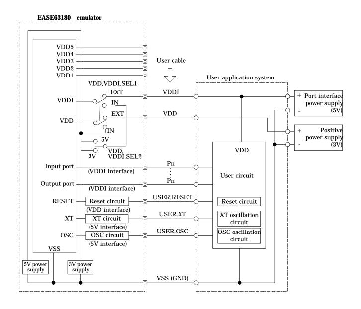
Figure 3-2 Power Supply Interface Example
