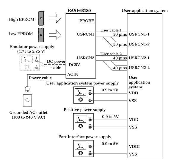
Figure 3-1 Connections for Evaluation
