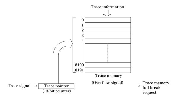
If trace memory full breaks are enabled, overflow during real-time emulation of the trace pointer, a 13-bit counter, produces a break request of this type.
