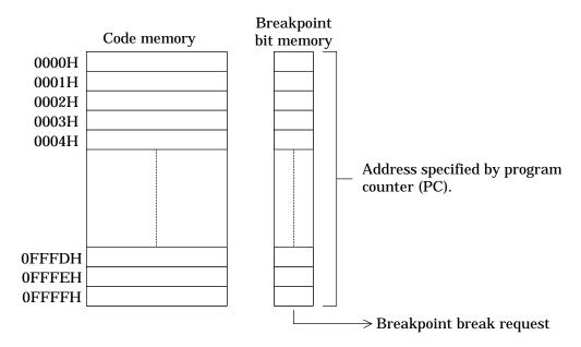
If these breaks are enabled, execution of the instruction at that address produces a break request of this type.
