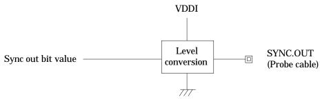
A built-in voltage conversion circuit converts the sync out (SYNC.OUT) signal "H" level to VDDI, the port interface power supply voltage (0.9 to 5 V), for output.
