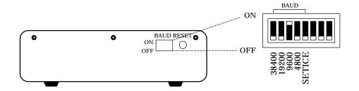
Figure 2-22 BAUD Switch
