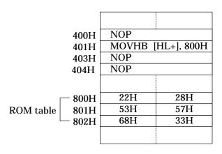
Specifying a ROM table address of 800H produces a break one instruction after the MOVHB [HL+],800H instruction at address 401H, that is, after the NOP instruction at address 403H.
