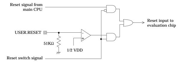
A built-in voltage conversion circuit converts the user cable reset (USER.RESET) input to the internal "H" level from VDD, the positive power supply voltage (0.9 to 5 V).
