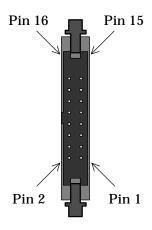
**Probe Connector Pin List**
