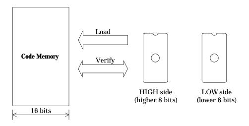
Figure 2-5 Data Operations between Code Memory and EPROMs
