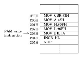
Specifying an address of any, a comparison value of 3, and a count of 1 produces a break one instruction after the once execution of the MOV [HL], A instruction at address 203H, that is, after the INCB HL instruction at address 204H.
