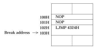
The address 103H never produces an address break.
