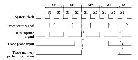
Figure 2-16 Trace Input Timing
