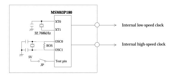
Figure 2-18 Crystal Board Circuits
