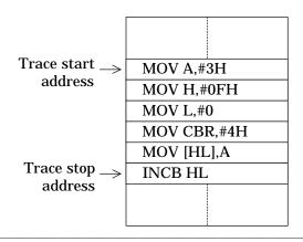
Tracing covers from the MOV A,#3H instruction at the start address through to the MOV [HL],A instruction preceding the stop address.
