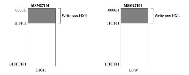
Figure 2-2 Address Ranges for MSM27101
