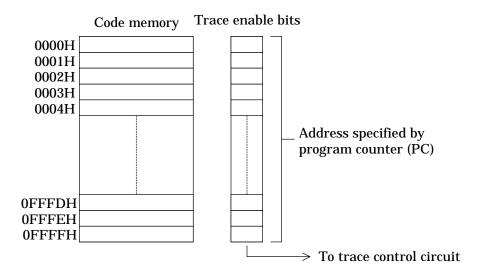
Figure 2-9 Trace Enable Bits
