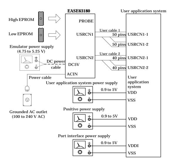
Figure 3-4 Connections for Emulation
