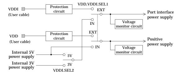
Port/positive power supply switch 1 (VDD+VDDI.SEL1) simultaneously switches VDDI and VDD between internal and external sources. Port interface power supply switch 2 (VDDI.SEL2) switches the internal VDDI source between 5 and 3 V.
