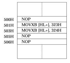
If external memory address 324H contains 55H, specifying an external memory address of 324H, a comparison value of 55H, and an access parameter of read only produces a break one instruction after the MOVXB [HL+],324H instruction at address 503H, that is, after the NOP instruction at address 505H.
