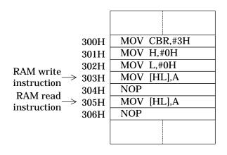
Specifying an address of 300H and a count of 2 produces a break one instruction after the MOV [HL], A instructions at addresses 303H and 305H, that is, after the NOP instruction at address 306H.
