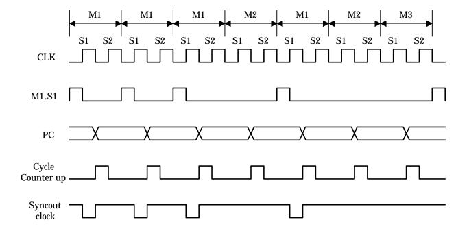
Figure 4-2 Cycle Counter/Sync Out Timing Chart
