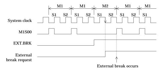
Figure 2-13 External Break Input Timing
