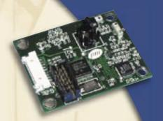
The TCM5 is the ultimate in compass modules, providing ultra precise heading information in any orientation. The first of its kind, this small, compact module provides for a full 360° rotation and complete flexibility, allowing it to be mounted in multiple orientations and positions. These advantages make the TCM5 the choice for applications that require the highest accuracy and performance anywhere in the world.
