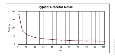
System designers need to balance electronic chopping frequency with emitter modulation depth, detector sensitivity and detector noise level which all decrease with increasing chopping frequency, but not at the same rate. The optimum electronic chopping frequency is chosen to maximize signal-to-noise ratio.
