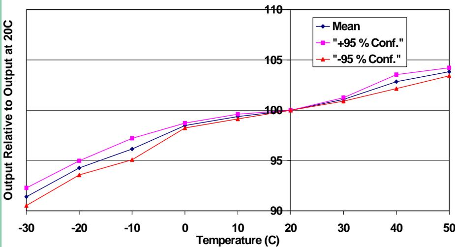
Figure 3 shows the variation in sensitivity caused by changes in temperature expressed as ppm gas equivalent.
