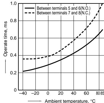
**4. Reverse time vs. ambient temperature characteristics**
