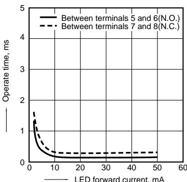
**11. LED forward current vs. reverse time characteristics**
