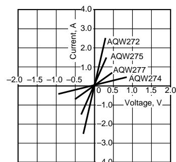
9.-1 Off state leakage current
