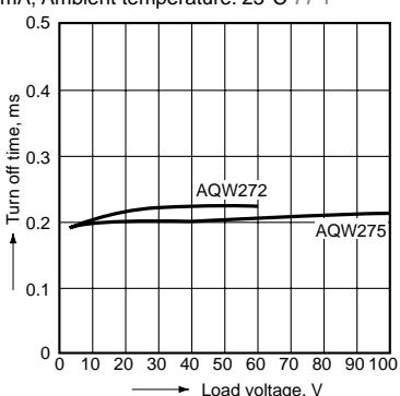
14.-2) Load voltage vs. turn off time characteristics
