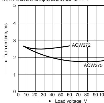
12.-2 Load voltage vs. turn on time characteristics
