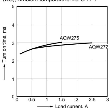
13.-2) Load current vs. turn on time characteristics
