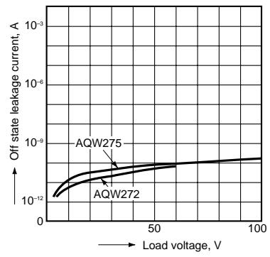
9.-2 Off state leakage current
