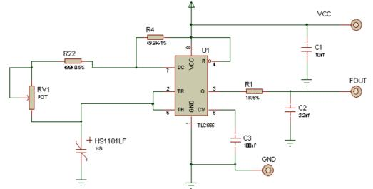
Note: R22=499k / R4=49.9k / R1=1 k / RV1=50 k potentiometer / C1=10nF / C2=2.2nF / C3=100nF
