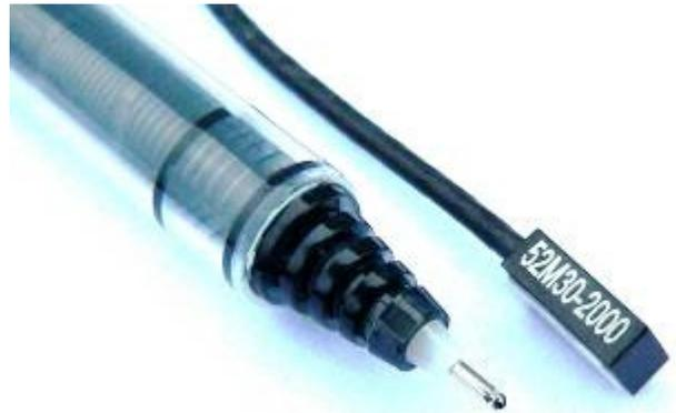
The **Model 52M30** accelerometer has an advanced piezoresistive MEMS sensing element which offers excellent dynamic range and stability. This unit features a full bridge output with an operating temperature range from -40 to 121 °C. A slight amount of gas damping provides outstanding shock survivability and a flat amplitude response to 7kHz.
