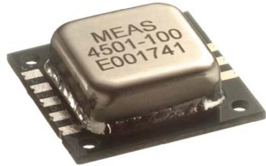
The **Model 4503** is an economical board mountable accelerometer with micro-g resolution. The output is signal conditioned and temperature compensated and offers an optional 2.5V reference for single-ended or differential output measurements. The model 4503 is available in ranges from  $\pm 2g$  to  $\pm 200g$  with a frequency response up to 1500Hz. The gas damped MEMS sensing element provides stable long-term performance.
