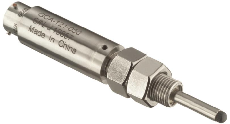
Internal construction prevents the core and shaft from rotating as they move longitudinally. Units terminating into connectors allow for easy cable replacement if damage should occur. Installation and adjustment are facilitated by external threading; locknuts are provided.
