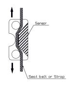
FSO (5KN): 1.5mV/V FSO (16KN): 2mV/V
