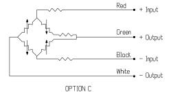
Electrical in: 25 mA max. FSO: 0.5 to 4.5V NL: < ± 0.5%FS0 Electrical out: short circuit
