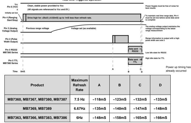
Real-time or triggered operation allows users to take advantage of a few functions unavailable during free run mode. When operating in triggered mode, an unfiltered maximum refresh rate can be achieved. This triggered operation allows users to range targets moving away from or closer to the sensor faster than 240mm/s.
