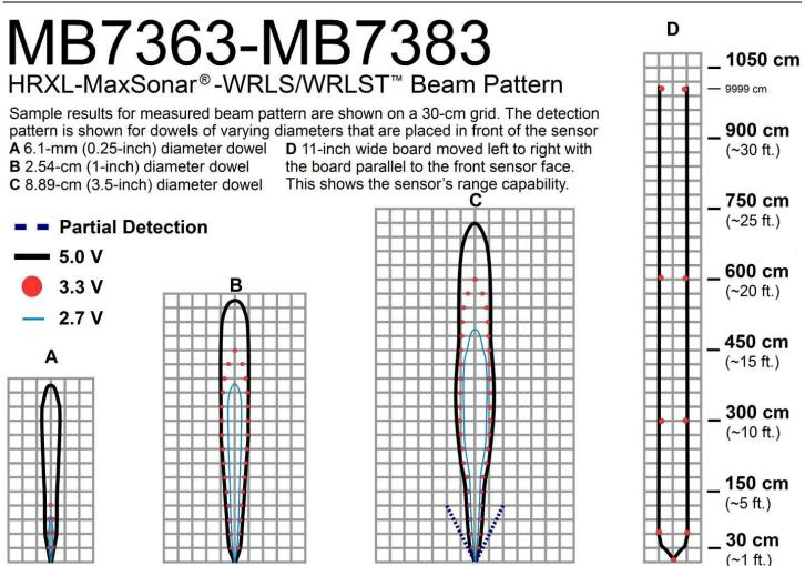
Beam Characteristics are Approximate Beam Pattern drawn to a 1:95 scale for easy comparison to our other products.
