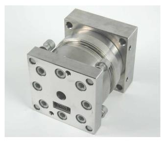
Fig. 1: Back view of crash force measuring element with 9 pin D-Sub connector
