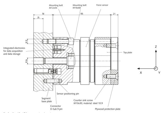
Fig. 2: SmartCrash® force measuring element
