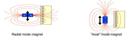
The orientation of the north and south poles is arbitrary, and the embedded software is highly tolerant of the magnet geometry so that rectangular bar magnets or cylindrical magnets can be used equally well. Cylindrical magnets in the axial mode are particularly attractive because the magnetic field is symmetrical with respect to rotation about the center axis without loss of position accuracy.
