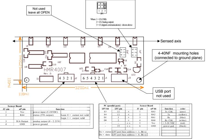
Figure 1 – Sensor board layout and connector pin designations
