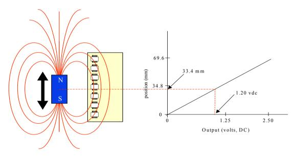
Figure 2. Position sensing example.
