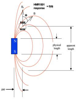
As the gap between the magnet and the sensor array increases, the apparent length of the magnet increases as well. A general rule of thumb for a cylindrical bar magnet is that the apparent length will increase by the amount of the gap. A twenty-five millimeter long magnet for example will appear to be thirty-five millimeters long at a gap of 10 millimeters. Since magnetic fields are highly nonlinear and subject to the exact geometry and properties of the material, this is only a general guide.
