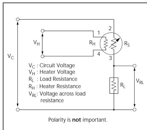
Fig 2. Standard circuit
