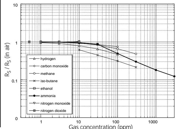
Fig 3. Sensitivity characteristics
