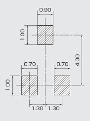
Note 1) The sensor center is located within the  $\phi$ 0.3mm circle.
