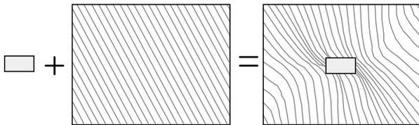
Ferrous Object + Uniform Magnetic Field = Field Disturbance
