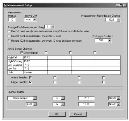
Figure 25. Measurement Setup Screen
