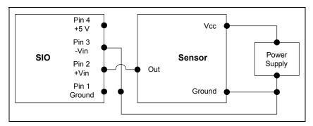
Figure 18. Externally Powered Sensor Connections
