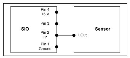
Figure 19. Current Sensor Connections
