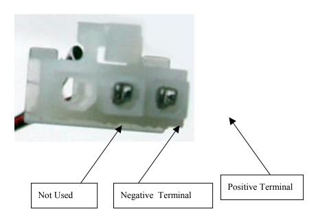
Figure E4. Pin Connection Diagram
