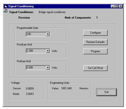
Figure B5. SIO Bridge Signal Conditioning
