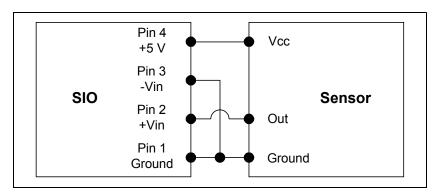
Figure 17. Internally Powered Sensor Connections
