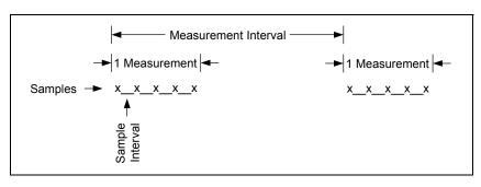
Figure 26. Samples and Measurements
