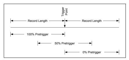
Figure 27. Pretrigger Fraction Options
