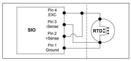
Figure 21. 3-wire RTD Sensor Connections
