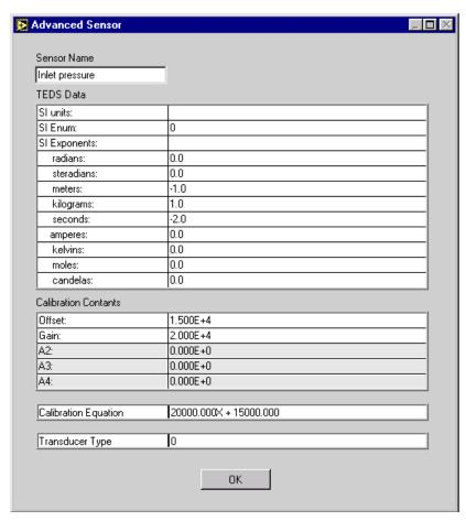
Figure C3. Advanced Sensor Screen
