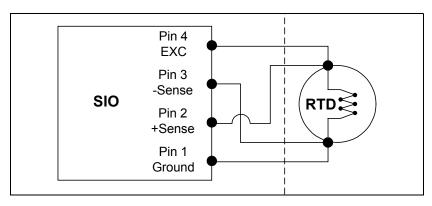
Figure 20. 4-wire RTD Sensor Connections
