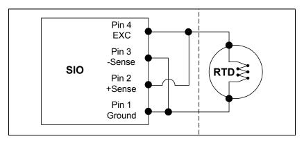
Figure 22. 2-wire RTD Sensor Connections
