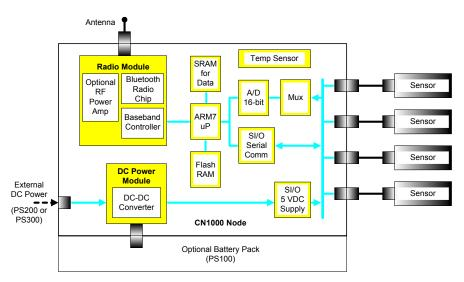
Figure 16. CrossNet Node Internal Architecture
