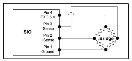
Figure 23. Bridge Sensor Connections
