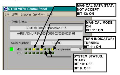
When the circle is completed, the following Gyro View BIT status should be displayed indicating the unit has made a full turn and is applying the estimated calibration. You should stop the rotation motion once the system status bits show the unit has reinitialized.
