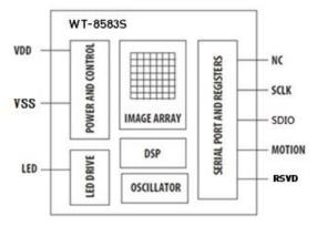
Figure 7. Block diagram of WT-8583S optical mouse
