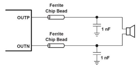
Ferrite Bead Filter to Reduce EMI
