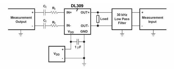
Notes:(1) CI was Shorted for any Common-Mode input voltage measurement;(2) A 33-uH inductor was placed in series with the load resistor to emulate a small speaker for efficiency measurements;(3) The 30-kHz low-pass filter is required even if the analyzer has an internal low-pass filter. An RC low pass filter (100 W, 47 nF) issued on each SUNSTAR单片机专用电路 http://www.icasic.com/ TEL: 0755-83387030 FAX:0755-83376182 E-MAIL:szss20@163.com output for the data sheet graphs.
