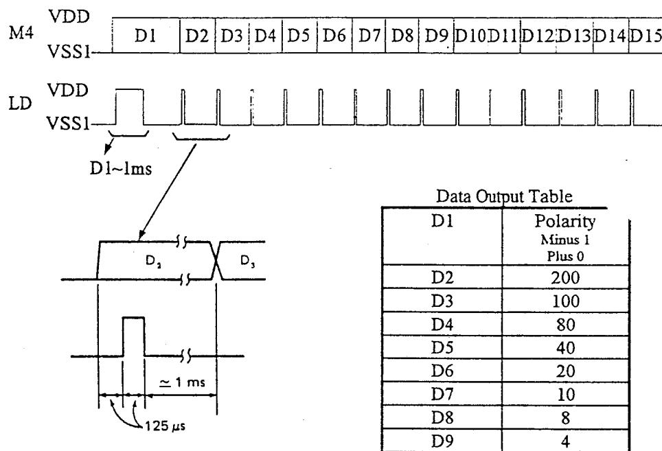
Note: (1) Data "1" is V<sub>DD</sub> level and "0" is V<sub>SS1</sub> level.
