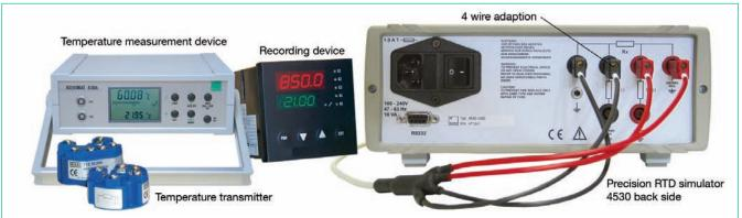
Calibration of temperature measurement, temperature regulators, head transmitters etc. in production
