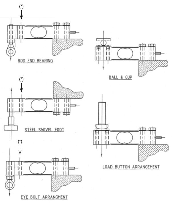
(\*) Note: Mounting using the 'inboard' hole is also acceptable
