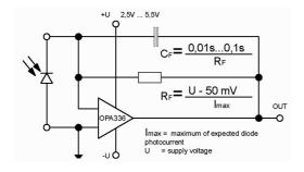
The adjacent design gives an example of a simple amplifier circuit. At the left side the photodiode is shown. The upper connection is the Cathode (isolated pin of the photodiode) and the lower connection is the Anode (usually grounded pin of the photodiode).
