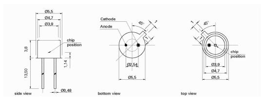
Selection code "18S" → TO18 Ni plated short housing, 5.6 mm diameter, 3.8 mm height two gold plated pins (Anode grounded and Cathode isolated). Not available with filters.
