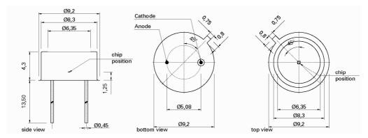
Selection Code "5" (photodiodes without filters) → TO5 Ni plated housing, 9.2 mm diameter, 4.3 mm height, two gold plated pins (Anode grounded and Cathode isolated).
