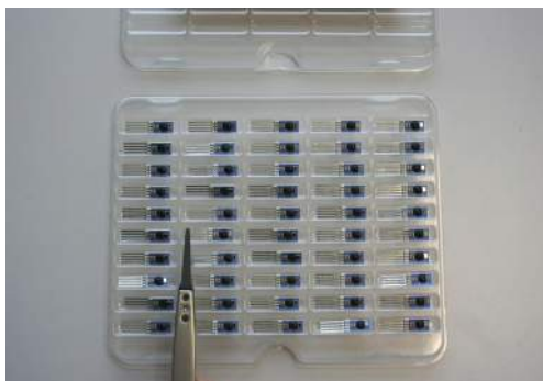
3. Take the sensors from the blister with plastic tweezers
