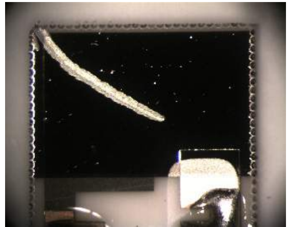
Sensor with a scratch
