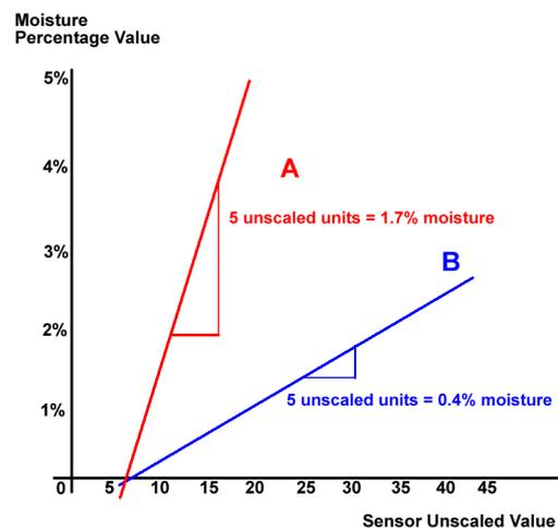
step (see line 'A', Figure 3). The ability to select the fundamental measurement technique allows the user to choose the technique that most flattens the relationship between unscaled values and moisture (see line 'B', Figure 3). The mathematical algorithms employed in the sensor have been specially devised to respond in a different manner dependent on the material. They will all give a stable linear output, however line 'B' in Figure 3 will give better accuracy and tighter precision.
