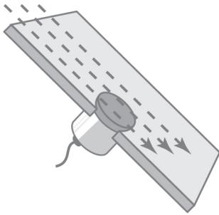
**Figure 1: Material Flow over a Moisture Sensor**
