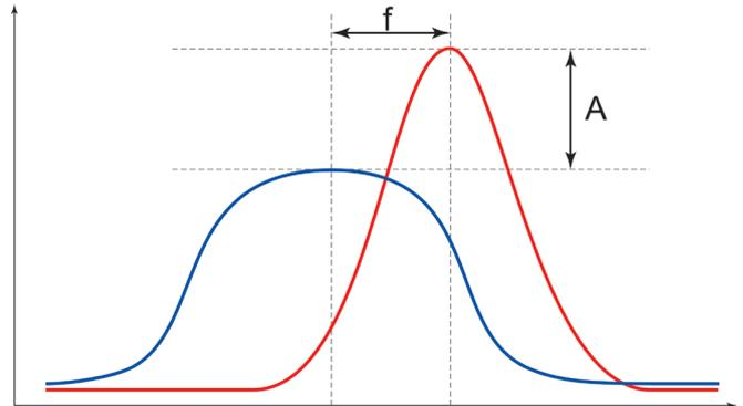
The latest breakthrough allows the sensor to measure, with digital accuracy, both the frequency and the amplitude responses of the microwave signal. These two measurements are then precisely combined using mathematical formulae to offer the user a choice of measurement modes. In practice, the user may now select from either Standard Mode (frequency shift technique) or two new modes that may be selected dependent on the material to give the best possible results.
