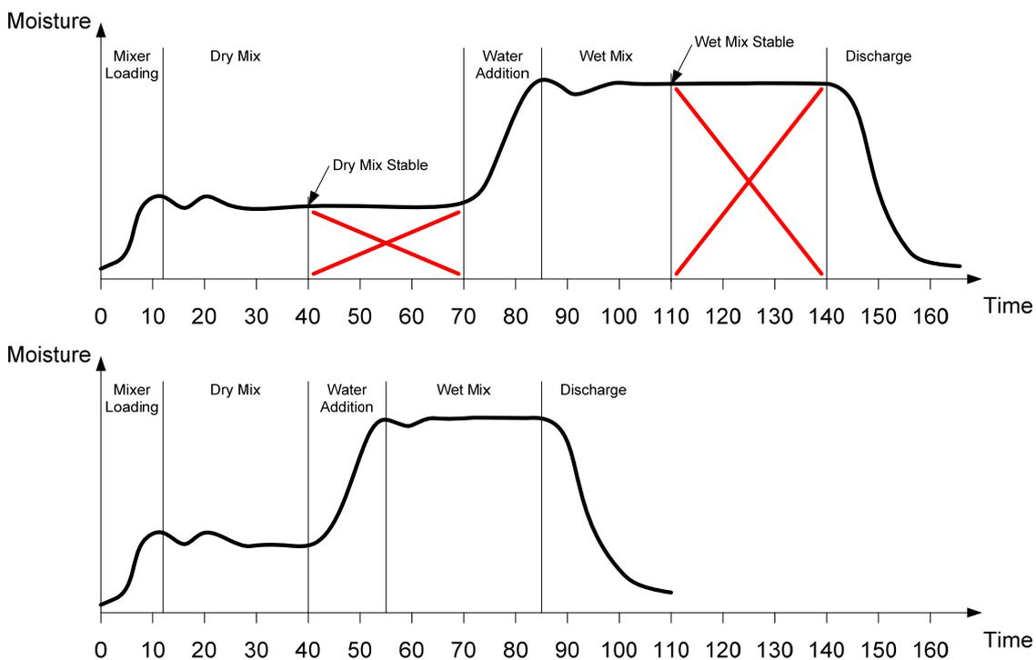
Figure 15: Extending the mix times for calibration
