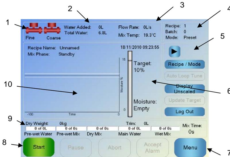
**Figure 2: The Overview Screen of the Hydro-Control VI**
