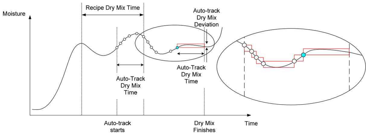
**Figure 28: Mix trace showing the Auto-track function**
