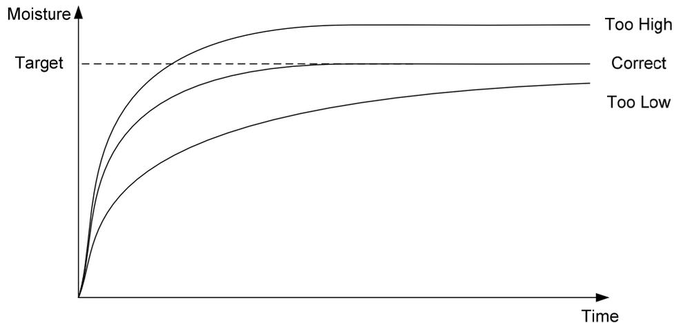
**Figure 23: The effect of changing the Proportional Gain**
