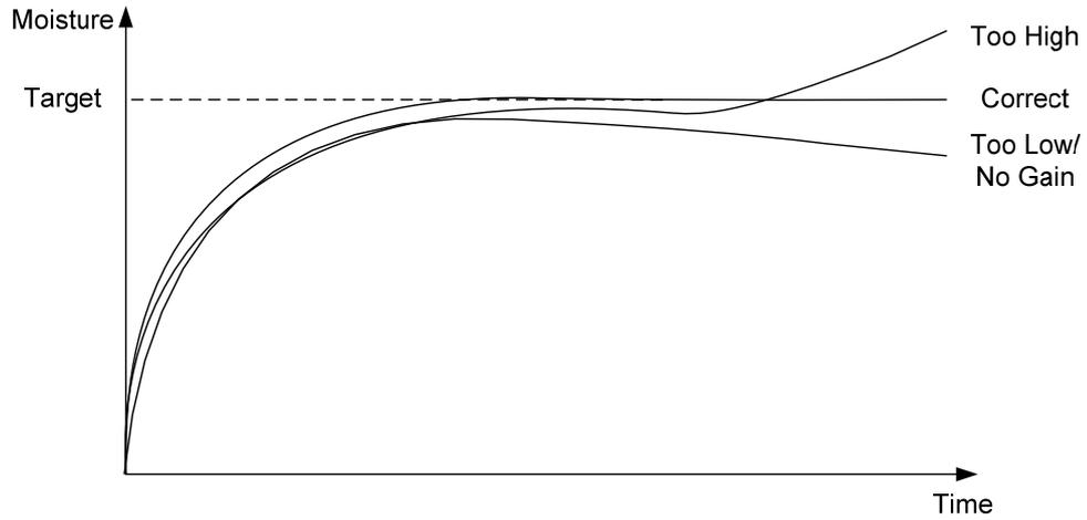
**Figure 24: The effect of changing the Integral Gain**
