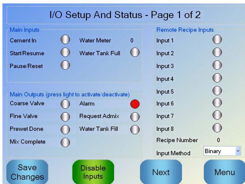
Figure 30: Page 1 of the I/O setup and status screen
