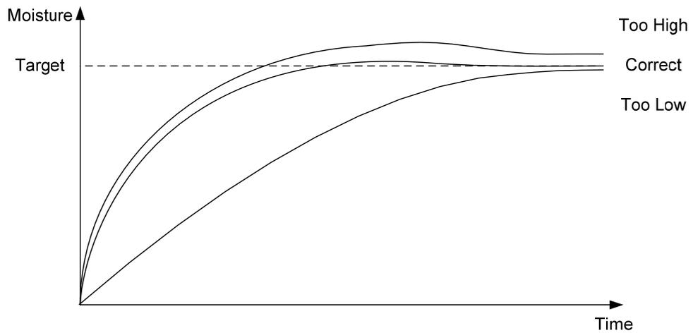
**Figure 25: The effect of changing the Derivative Gain**
