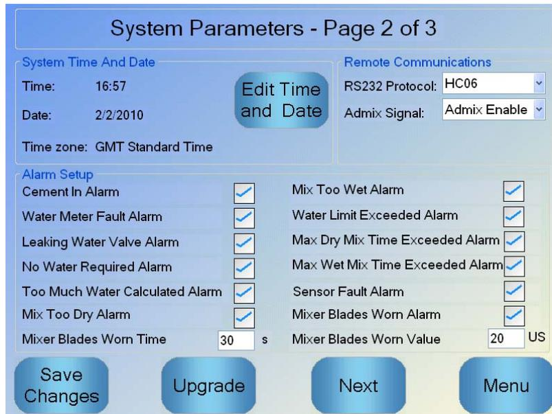
Figure 29: Page 2 of the System Parameters screen
