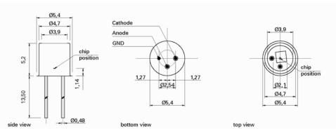
Selection code "18ISO90"  $\rightarrow$  TO18 Ni plated housing, 5.6 mm diameter, 5.2 mm height three gold plated pins (Anode and Cathode isolated, additional third pin for optional grounding of the body).
