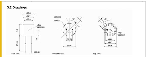
Selection code "18"  $\rightarrow$  TO18 Ni plated housing, 5.6 mm diameter, 5.2 mm height two gold plated pins (Anode grounded and Cathode isolated).
