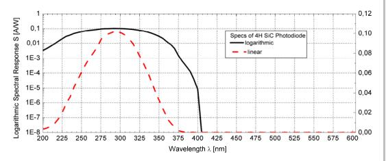
The curve's maximum is at approximately 300nm. The response falls down to 10% of maximum at 215nm, (UVC edge) and 365nm, (UVA edge). Unfiltered SiC can be used for any UV measurements where the whole UV band needs to be measured or a quasi monochromatic UV source (such as low pressure lamps) is controlled.
