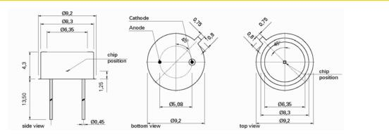
Selection Code "5" (photodiodes without filters)  $\rightarrow$  TO5 Ni plated housing, 9.2 mm diameter, 4.3 mm height, two gold plated pins (Anode grounded and Cathode isolated).
