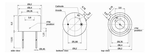
Selection Code "5" (photodiodes with filters)  $\rightarrow$  TO5 Ni plated housing, 9.2 mm diameter, 6.6 mm height, two gold plated pins (Anode grounded and Cathode isolated).
