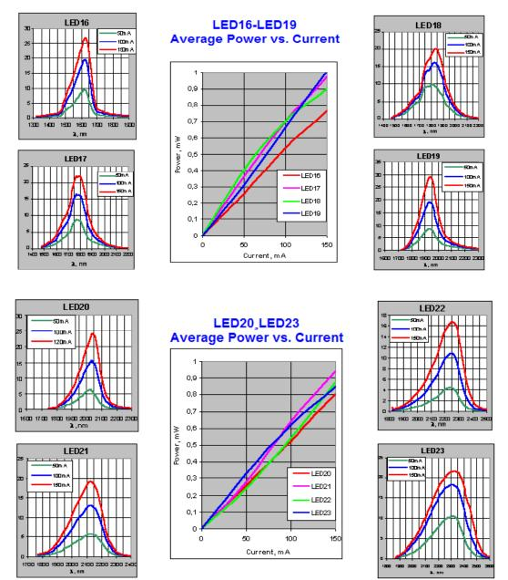
Full power can be measured correctly only by use of integrated sphere. Power of our LED practically doesn't decrease with increase of modulation frequency up to 10 MHz. Spectral intensity is shown in arbitrary untis.
