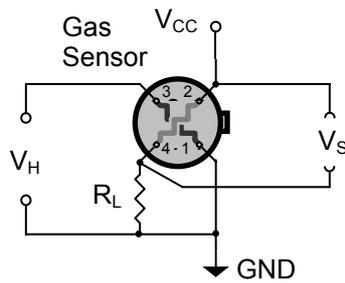
Figure 3: MiCS-5525 with measurement circuit (top view)
