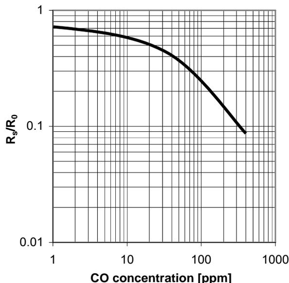
Figure 2:  $R_s/R_0$  as a function of CO concentration at 40% RH and  $25 \text{ }^\circ\text{C}$ , measured on an engineering test bench
