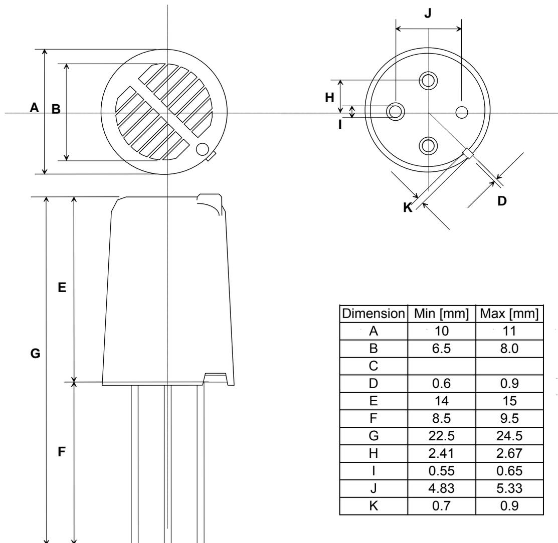
e2v semiconductor gas sensors are well suited for leak detection and applications requiring limited accuracy. Their use for absolute gas concentration detection is more complicated because they typically require temperature compensation, calibration, and sometimes as well, humidity compensation. Their base resistance in clean air and their sensitivity can vary over time depending on their environment. This effect must be taken into account for any application development (1102-1.0).
