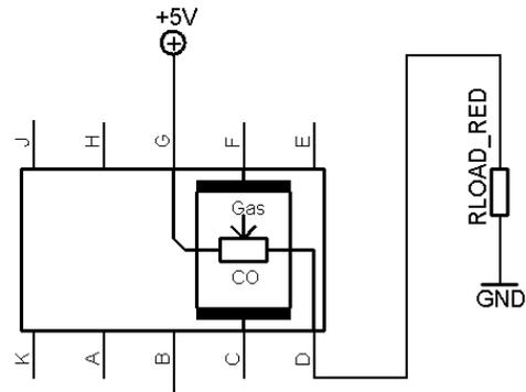
**Figure 3: MiCS-5524 with measurement circuit (top view)**
