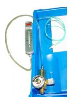
• Field Calibration Kits are available and consist of the following: (See page 3 for part numbers) one tank with approx 8 hour supply of 99.8% N<sub>2</sub> one tank with approx 8 hour supply of CO<sub>2</sub> flow meter - 0 to 500 ml/minute range (Includes 2 plastic hose barbs) pressure regulator w/flow control valve - 0.3 L/min two plastic interconnect calibration gas tubes carrying case - 23 x 9 x 4.5 inches
