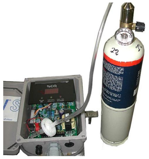
See the **specification sheet** for the specific full scale **Model 2166** you are calibrating and find the response scale chart that shows both the 0 to 5 volt and 4-20 mA outputs as a function of gas concentration. As an example, a 1%  $CO_2$  full scale unit should have a 2.50 volt output or 12.0 mA output for certified 0.5%  $CO_2$  span gas.
