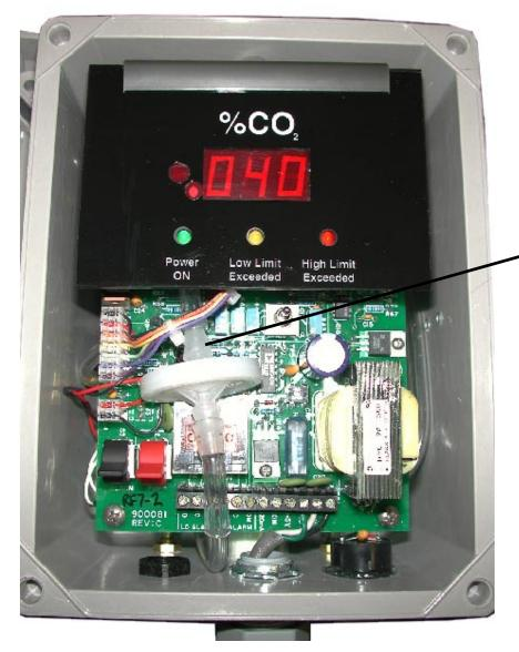
**INLET** side of Hydrophobic filter. See **Application Note A24** for complete gas calibration instructions.
