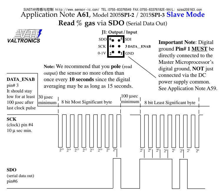
Decimal 500 = implied 5.00% gas = binary 0000 0001 1111  $0100 = 2^8 + 2^7 + 2^6 + 2^5 + 2^4 + 2^2 = 500$  decimal Divide decimal value by 100 to equal % gas reading on a Model 2005SPI-2 or 2015SPI-3 sensor.
