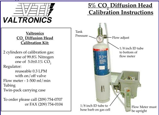
Gas calibration should be done a minimum of once every six months (at least ZERO calibration).
