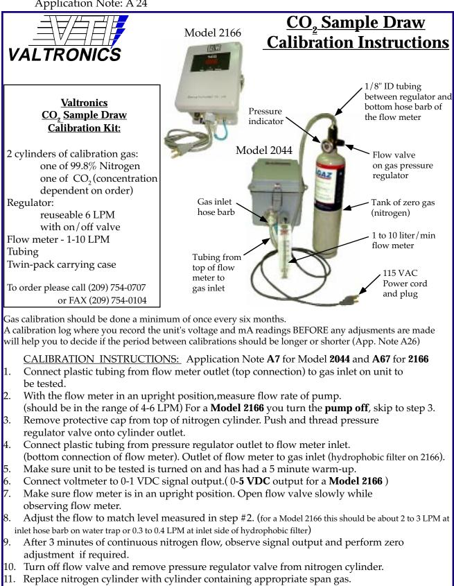
(Near mid-range value - Example: for 0 - 3000 ppm unit, use 1000 ppm or 0.1% span gas.)12. Open flow valve and observe signal output. (see scale data for voltage reading)
