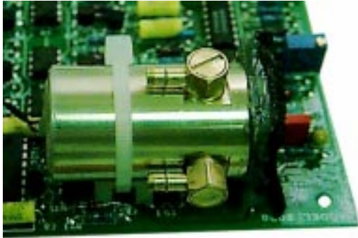
Adjustable 90° hose barb option on gas cell for lower profile
