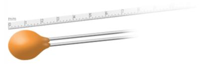
BetaCURVE Thermistor Series III are similar in construction to Series I except for the use of larger (30 AWG) copper leads. This allows the Dissipation Constant (D.C.) to be raised from 0.75mW/°C to 2.0mW/°C. Larger leads also facilitate easier handling during assembly operations. The Thermal Time Constant is raised to 14 seconds in air. Custom resistance values and tolerances are available upon request.
