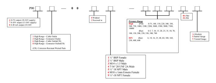
Examples: P9061-0002-7K5PSS = 0 to 5V output from 10 to 36V supply, cable outlet, welded '4' BSP male port, 7500 psi sealed gauge P9083-0023-10BAV = 4-20mA output from 10 to 36V supply, connector outlet, screwed in M14 male port, 10 bar vented gauge
