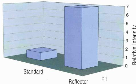
An optimized reflector design offers a gain of approx. 7 times in intensity on the optical axis.
