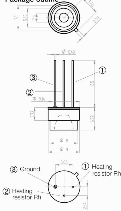
The IRSOURCE is a micro-machined electrically modulated thermal infrared emitter with a compact package, no mechanical moving parts and a long lifetime.
